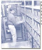
High density facilities emphasize shelving efficiency. Materials are sorted and shelved by size on specially designed units that stand 18 feet high. We use a special lift to retrieve volumes stored on the high shelves. Because of this, the storage portion of the facility is not open to the public. Instead, requested materials are delivered twice a day to Van Pelt, and once a day to the other Penn Libraries.
